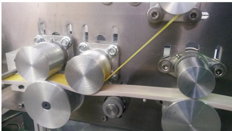
**T**hus, to meet various needs, Sterne proposes adhesive positioning on different silicone supports such as: sheets, molded plates, and profiles with widths ranging from 6 mm to 60 mm max, and a height of 20 mm max on different lengths of rings. Sterne offers also a standard adhesive range whose advantages are shear chemical agents and moisture strength for a wide panel of temperature brittleness.
